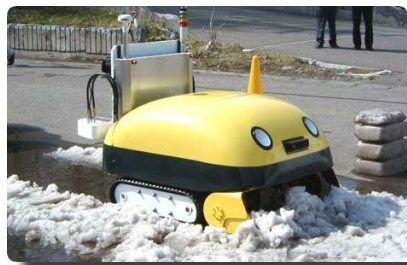
Yuki-Taro Autonomous Snow Plow Robot
